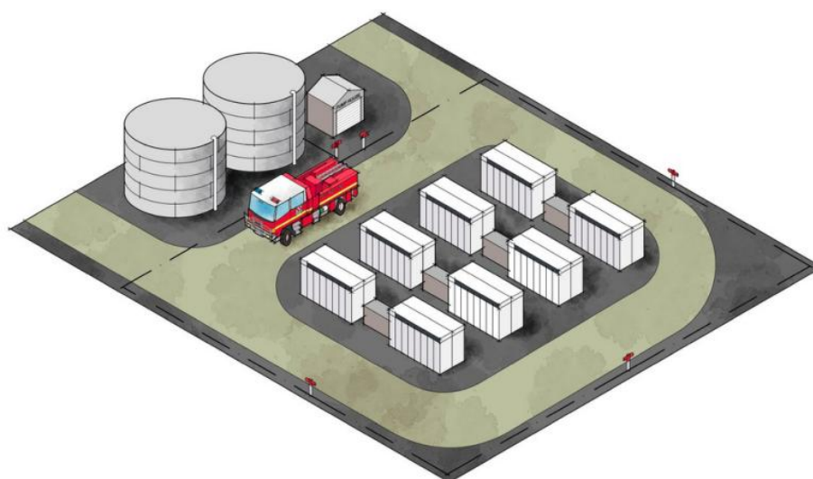
Plate 1: Best practice arrangement of fire service infrastructure for facilities with centralised battery energy storage systems with reticulated water supply meeting the performance requirements of AS 2419.1-2021: Fire hydrant installations .
