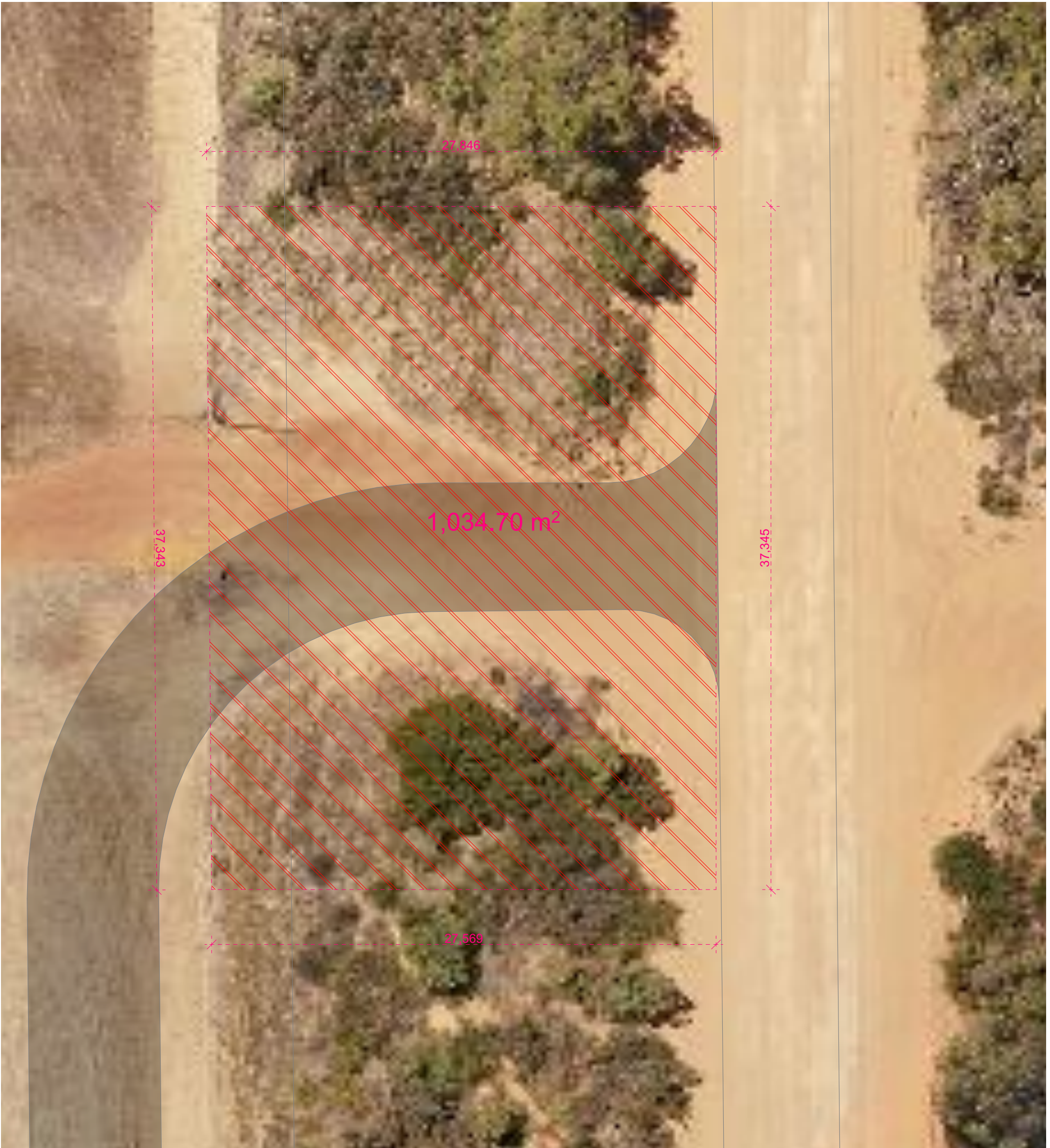
2 CLEARING - GILLINGARRA RD CROSSOVER 1:200
