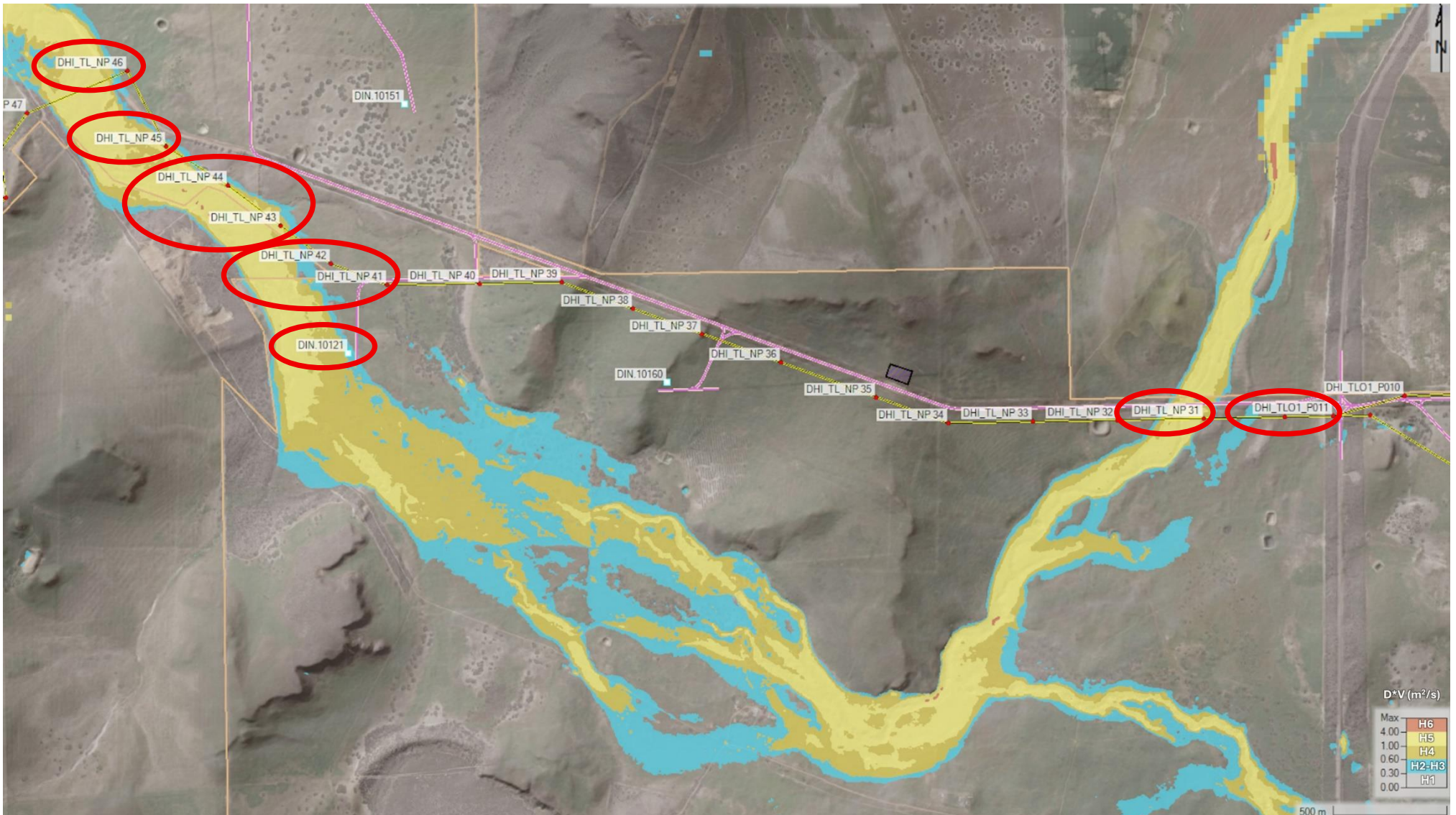
Figure 4-36: Maximum 1% AEP flood hazard for WTG and transmission towers in 1% AEP floodplain
