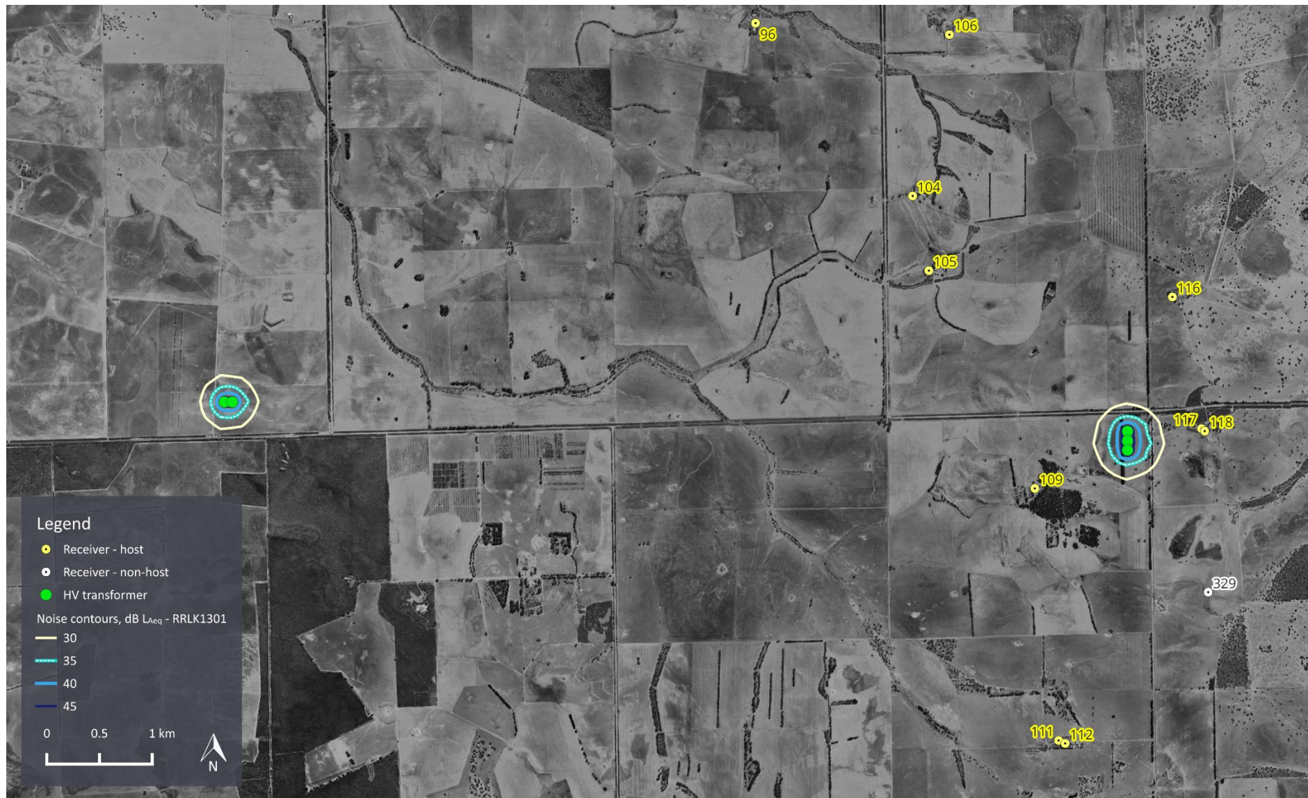
Figure 13: Additional substations predicted noise level contours
