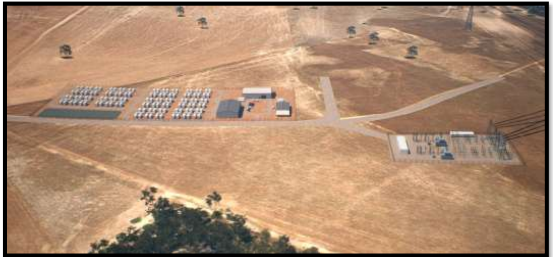
Figure 4: Visualisation of Harvest BESS and Substation
